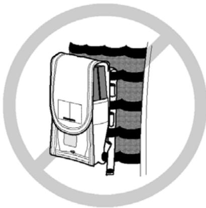
Figure 2. Wrong Pouch/Pocket Attachment.
